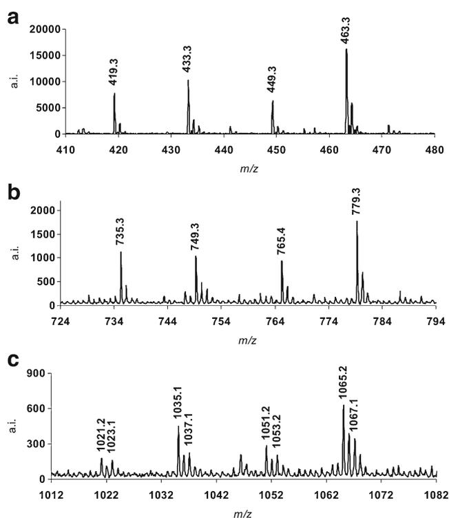
**Fig. 5** MALDI-TOF positive reflectron mode mass spectra of the anthocyanin-polyflavan-3-ol oligomers of “HyRed” cranberry fruit and spray-dried juice. (a) Anthocyanins  $[\text{M}]^+$ . (b) Anthocyanin linked to a single flavan-3-ol through a  $\text{CH}_3\text{-CH}$  bridge  $[\text{M}]^+$ . (c) Anthocyanin linked to a polyflavan-3-ol of two degrees of polymerization through a  $\text{CH}_3\text{-CH}$  bridge, containing either an A-type or a B-type interflavan bond  $[\text{M}]^+$  [69]
